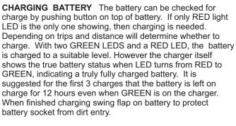
**Note WARRANTY** does not cover battery, if its not charged regularly, or left over time without at least one GREEN LED (of the two) illuminated. Never leave uncharged with just the RED LED showing.
