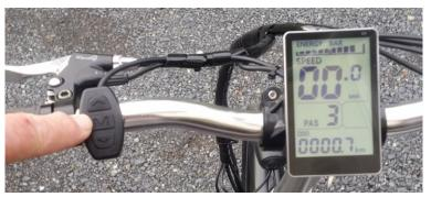
Electric Controller With battery key turned "ON"
